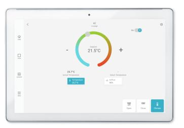
**Zone Temperature Set Point** (Only available if zone temperature sensors have been installed)
