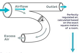
Diverted excess air leaves through a constant vent with 1 degree accuracy using iZone's advanced constant control algorithm.
